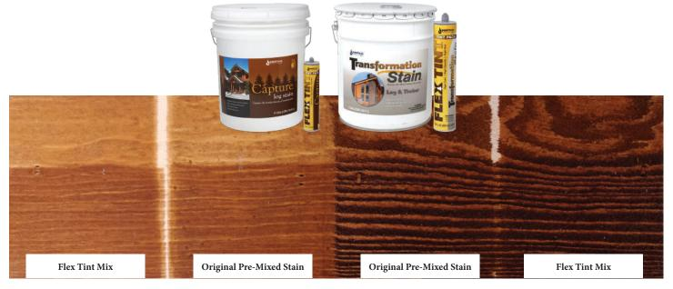
Top half has 1 coat. Bottom half has 2 coats. Left side was sanded smooth. Right side was blasted.
